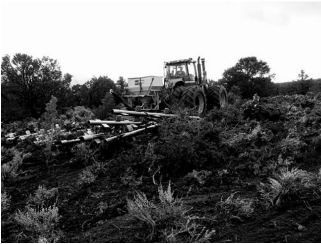
Figure 2. Photo of Dixie harrow courtesy of United States Department of Interior Bureau of Land Management, Richfield, Utah, USA.
